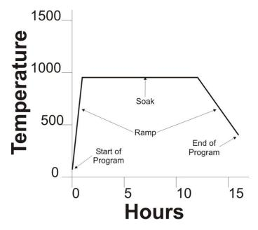
The annealing oven heats (Ramps up) to the annealing temperature. If cold glass is in the annealer, the ramp rate up is slow to prevent thermal shock and breakage. The glass is held at the annealing temperature long enough for the manufacturing stress within the glass to be released (Soak). The glass is then cooled (Ramps down) at a slow enough ramp rate so as not to reintroduce too much stress back into the glass.
